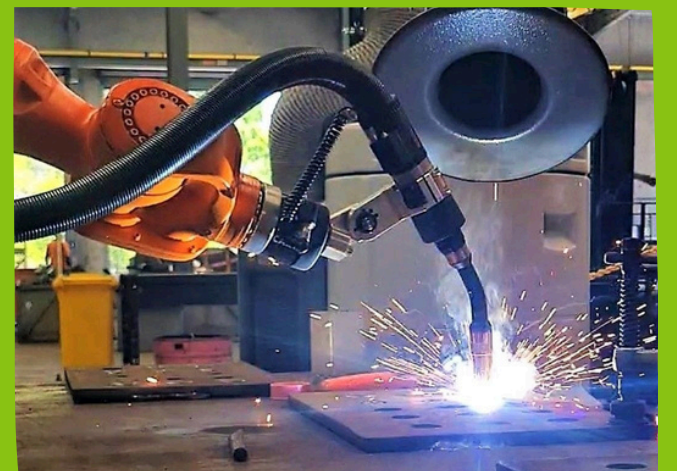
Local Exhaust Ventilation can extract solvent vapours & filter welding fume.
