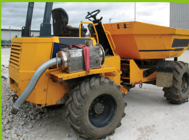
Diesel Engine Exhaust Filters can help protect against DEEs.
